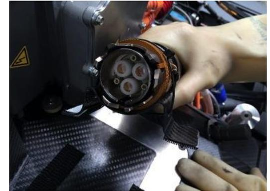
18. Inspect the mechanical state of the DC and AC cables(if existing)
