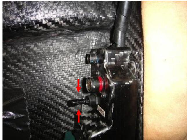
14. Go to P0 (Up) - Disconnect the 2 RESS low voltage connectors (red and blue)
