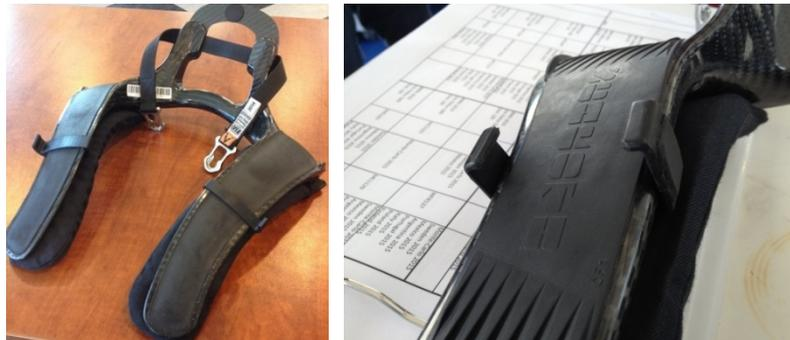
Figure 1 – HANS device with additional small brackets at the bottom of the HANS-yoke
