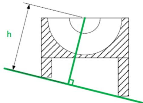
$h \geq 100\text{mm}$  must be respected for at least one cross section of the sump perpendicular to the crankshaft centreline
