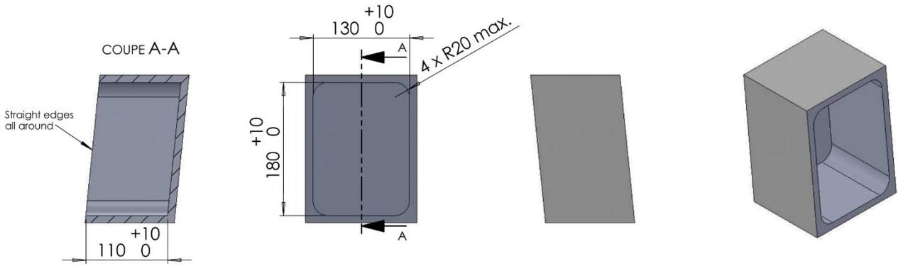
Any chamfer or radius above 5mm which would reduce these dimensions is not permitted.
