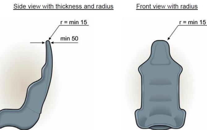
Figure 1. Geometry of upper section of seat backrest
