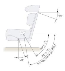
Figure 7 Side view to show recommended belt angles
