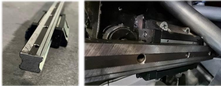
Caged Ball Linear Motion Guide attached to the steering column
