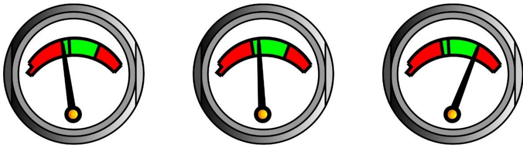
Extinguisher systems with a pressure gauge showing the above readings shall be considered OK
