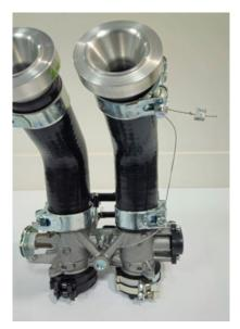
The engine will be considered non-compliant with Article 279B-4.14.2 if a broken seal is detected during an event.
