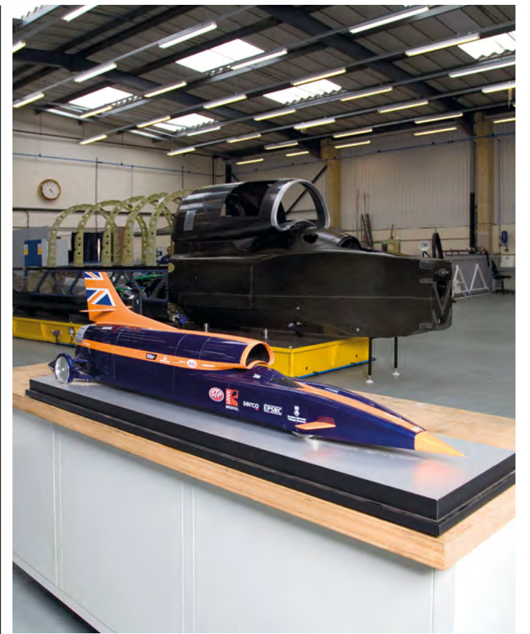
The car is a hybrid construction with the forward half made of carbon fibre and the rear section a metallic fabrication. To push Bloodhound through the 'K', the team may opt for a Jet over Rocket configuration
