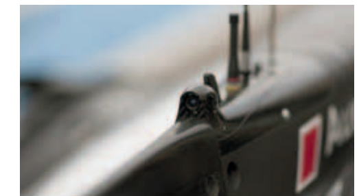
Audi has improved the safety and driver environment of its 330km/h R18 Le Mans Prototype racer (above) with this tiny high-tech rear-view OLED camera
