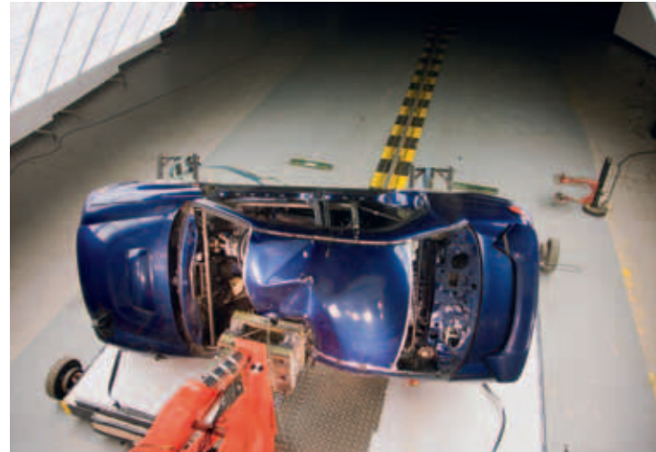
A series of near identical and precisely angled collisions in simulated roll-over accidents test the resilience and strength not only of the steel used in tubular cages fitted to competition cars, but also the quality and nature of the welds; a high-speed camera (below) freezes every detail; Mellor (right in picture, far right) inspects the set-up
