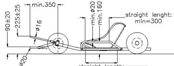
Lower attachments horizontal and parallel to the axis of the chassis
