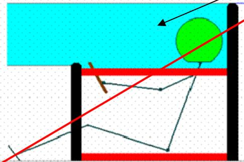
The shaded area shown on the left (plan view and side view) must be clear any edges of the bodywork or solar generators except in the cases shown in example 1 and 2 below. Any such edges can result in the injury to the driver's head in the event of accident including collision.
